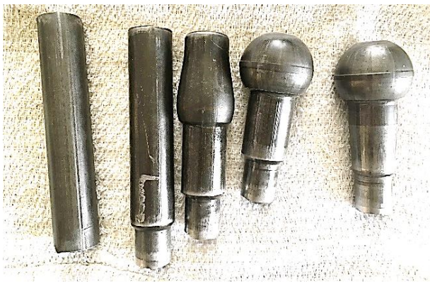
Figure F: Part Progression and Tool Layout provided by PRF Manufacturing Roseville MI
